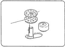
Draw thread from spool through bobbin Pull end of thread through hole in Place bobbin as shown.
